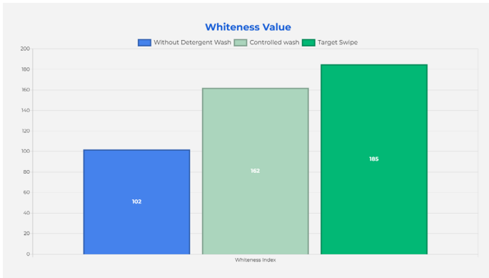
Whiteness Retention – 30 Washes at 30°C (KLORIMAX™ Target Swipe vs. Alkaline Institutional Detergent vs. Control)
